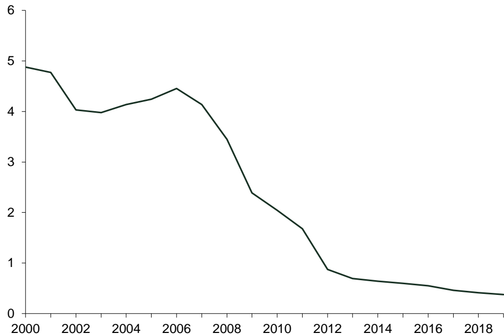
Figure 2.1 Evolution of global average solar PV module prices between 2000 and 2019 (in US$ per Watt)
